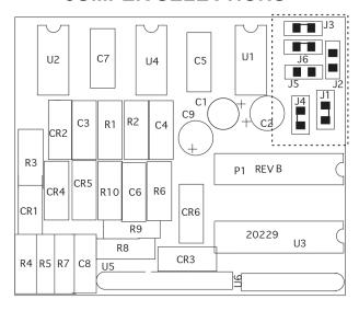
If the unit has the millivolt input bd.# 20229, A & B inputs can be separately solder jumper programmed to accept either a low millivolt or 4-30 V input. Each unit shipped is programmed according to part number. If solder jumpers are made, the part number should be modified to reflect the changes made.
