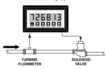
The MINI-Batcher is the central controller for this simple water batching application. The batcher accepts pulse inputs from a turbine flowmeter and uses relay(s) to control a solenoid valve.
