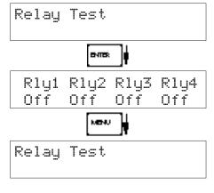
Press Enter to test the relays.
