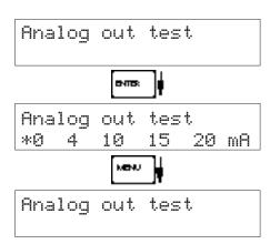
Press Enter to test the analog output.
