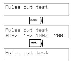
Press Enter key to test the pulse output.
