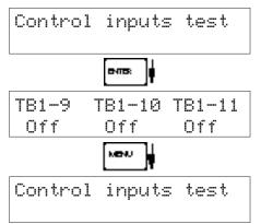
Press Enter to test the control inputs.
