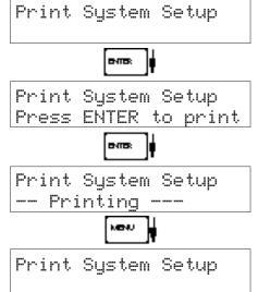
Press enter key to enter print system setup submenu
