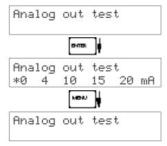
Press Enter to test the analog output.
