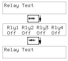
Press Enter to test the relays.
