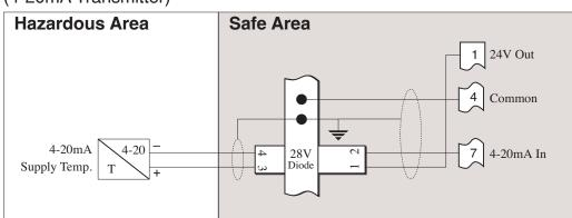
Return Temperature Input (4-20mA Transmitter)
