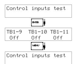
Press Enter to test the control inputs.
