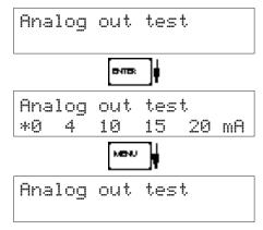
Press Enter to test the analog output.
