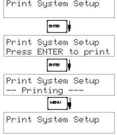
Press enter key to enter print system setup submenu
