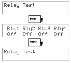
Press Enter to test the relays.
