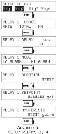
Select the desired Relay for setup. (Relays 3 & 4 Optional)
