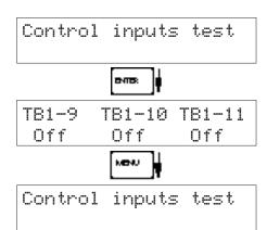
Press Enter to test the control inputs.
