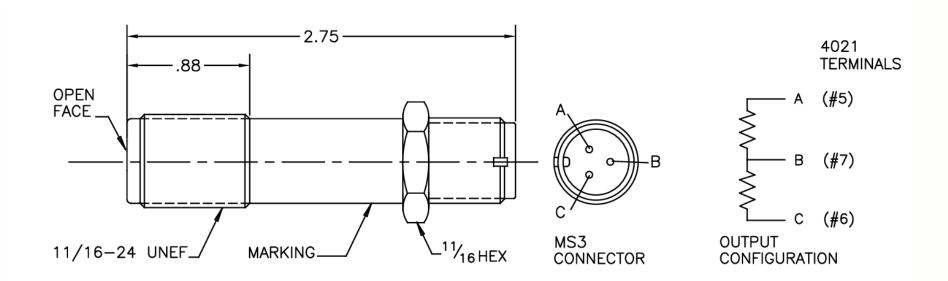
THIS SPECIAL PICKUP IS DESIGNED TO WORK IN VERY NOISY ENVIRONMENTS AND MUST BE USED IN CONJUNCTION WITH THE 4021 TYPE II SERIES PREAMP.
