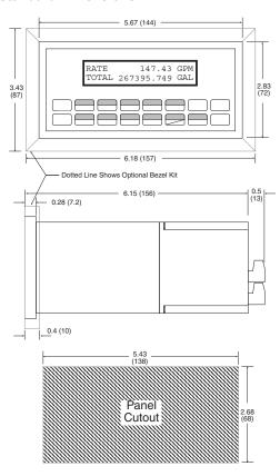
Fig. 2: Wall Mount ("W" mounting option) Dimensions
