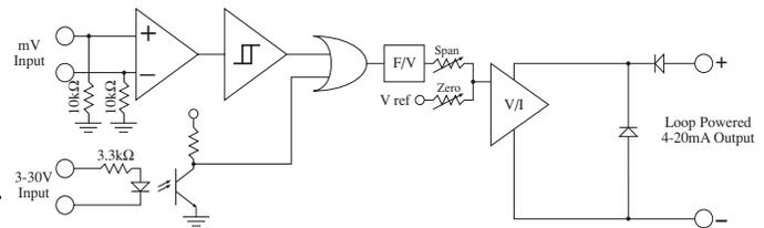
**Typical Application Magnetic Pickup Input**
